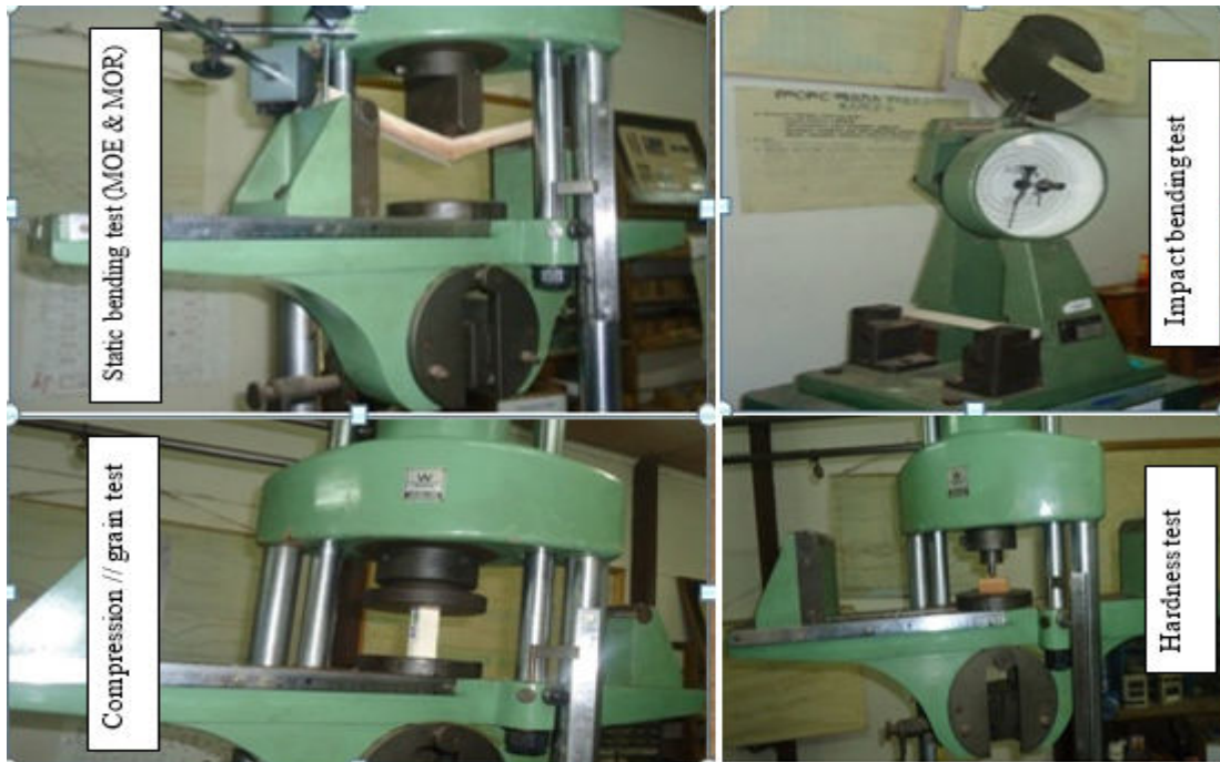
Figure 5: Mechanical properties tests using Universal Testing Machine (UTM)
