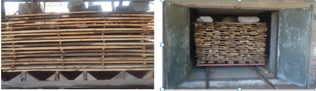
Figure 3: Stacked lumber of A. melanoxylon for air seasoning (a) and for kiln seasoning (b)
