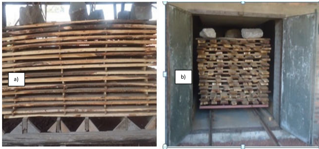
Figure 29: Pictures showing lumber stacked for air drying (a) and kiln seasoning (b) of A. melanoxylon lumber
