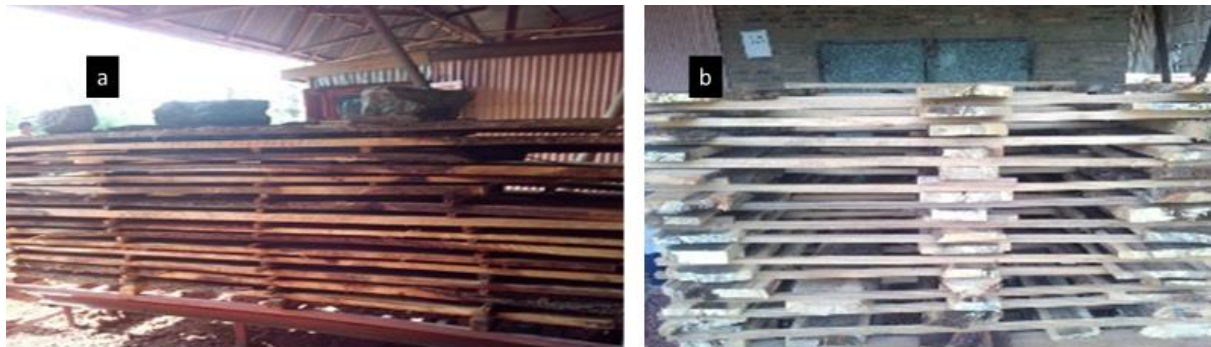
Figure 4 Air (a) stack and kiln seasoning stack (b) (Kiln seasoning stack before entering the kiln chamber)
