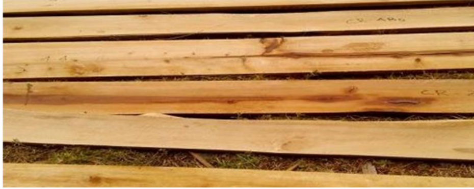
Figure 3 Surface appearance of C. equisetifolia boards
